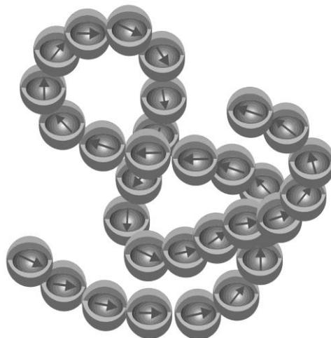
Fig.3: Suggested schematic view on 1D chain-like structures formation in silica coated iron nanoparticles.
